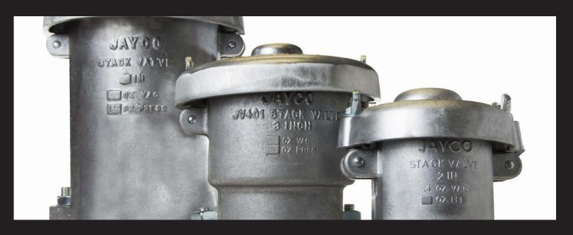
THE PURPOSE OF THE VENT VALVE IS TO WORK IN TANDEM WITH THE THIEF HATCH TO MINIMIZE THE ESCAPE OF LIGHT ENDS OF CRUDE IN LEASE STORAGE BY MAINTAINING A PRESSURE ON THE TANK. STACK VALVES INSTALL ATOP A VER-TICAL PIPE. PRESSURE FROM THE VESSEL IS VENTED TO ATMOSPHERE WHILE A VACUUM ON THE VESSEL DRAWS OUTSIDE AIR THROUGH THE VALVE. OPTIONAL VENTING LEVERS ARE AVAILABLE FOR MANUAL VENTING. THE VALVE BODIES ARE ENGINEERED TO HAVE LOW IMPACT ON THE FLOW OF MEDIA THROUGH THE PIPE RUN.
