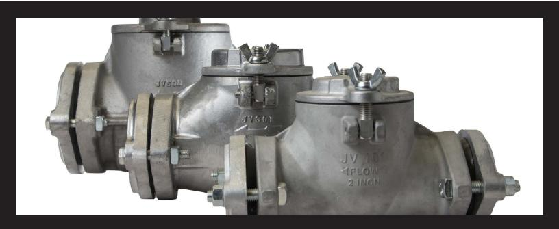
THE PURPOSE OF THE VENT VALVE IS TO WORK IN TANDEM WITH THE THIEF HATCH TO MINIMIZE THE ESCAPE OF LIGHT ENDS OF CRUDE IN LEASE STORAGE BY MAINTAINING A PRESSURE ON THE TANK. A VACUUM RELIEF FUNCTION IS ALSO STANDARD WITH OPTIONS TO CLOSE OFF FOR PREASURE ONLY. SLIP ON FLANGES AT EACH END ALLOWS FOR CON-NECTION TO THE HORIZONTAL PIPE RUN. THE VALVE BODIES ARE ENGINEERED TO HAVE LOW IMPACT ON THE FLOW OF MEDIA THROUGH THE PIPE RUN.
