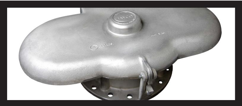
THE PURPOSE OF THE THIEF HATCH IS TO WORK IN TANDEM WITH THE VENT VALVE TO MINIMIZE THE ESCAPE OF LIGHT ENDS OF CRUDE IN LEASE STORAGE BY MAINTAINING A PRESSURE ON THE TANK. A VACUUM RELIEF FUNCTION IS ALSO STANDARD. THE THIEF HATCH PERMITS ACCESS TO THE CONTENTS OF THE TANK FOR SAMPLING AND GAUGING. THE JT-20.1 FEATURES A 20" OBLONG DRIP PAN TO CONTAIN DRIPPINGS AND GIVES THE OPERATOR A WORKSPACE FOR TOOLS.
