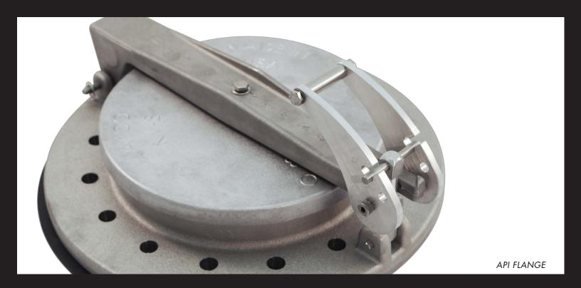
THE JAYCO NV-8 NON-VENT HATCH PROVIDES A VAPOR TIGHT SEAL WHILE GIVING THE OPERATOR ACCESS TO THE CONTENTS OF THE STORAGE TANK. THIS HATCH DOES NOT ALLOW VENTING TO THE ATMOSPHERE BUT DOES ALLOW GAUGING, SAMPLING AND MEASURING OF LEVELS. BOLT PATTERN COMES IN 16 HOLE API OR 8 HOLE ANSI 150 LB.
